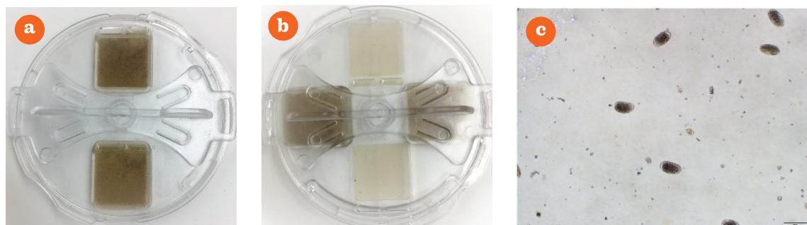
Fig 1. Mini-FLOTAC apparatus (a) loaded sample, (b) reading mode, (c) acquired image with Trichostrongyles type eggs, and Eimeria sp. oocysts.
